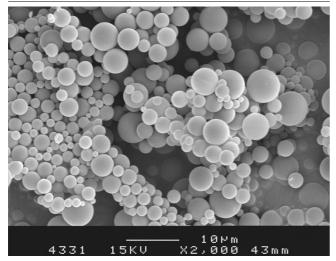
Scanning electron microscopy image of the microparticles.
