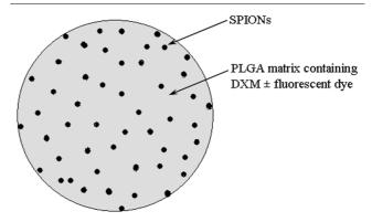
Schematic representation of a microparticle. DXM, dexamethasone 21-acetate; PLGA, poly(D, L-lactide-co-glycolide); SPION, superparamagnetic iron oxide nanoparticle.
