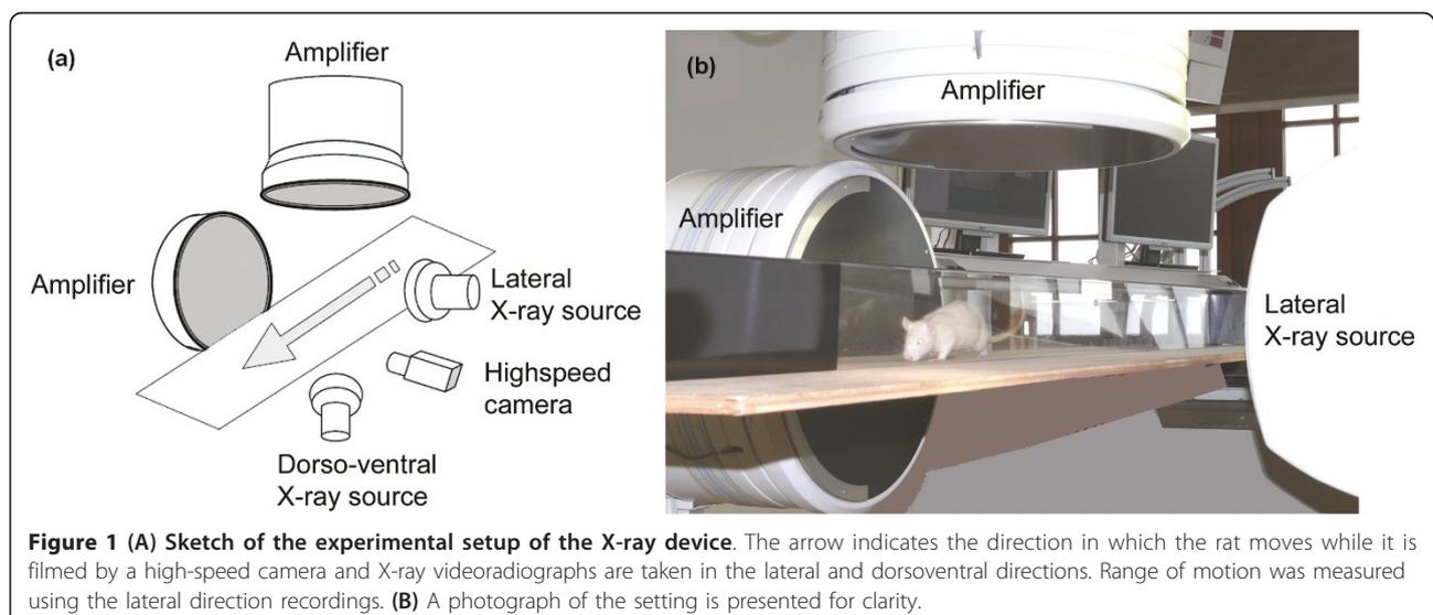
**Figure 1** (A) Sketch of the experimental setup of the X-ray device. The arrow indicates the direction in which the rat moves while it is filmed by a high-speed camera and X-ray videoradiographs are taken in the lateral and dorsoventral directions. Range of motion was measured using the lateral direction recordings. (B) A photograph of the setting is presented for clarity.
