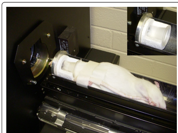
Figure 1 In vivo micro-CT imaging of a rat hind limb; anaesthetized rat on the scanner bed in supine position, with the hind limb secured in a customised leg fixative device (inset). Micro-CT, micro-computed tomography.
